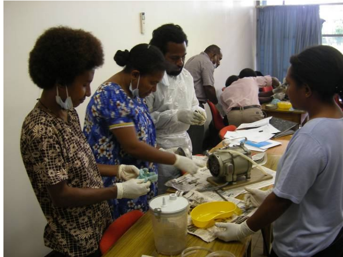
PNG Nurses learning how to change the oil in a suction pump
