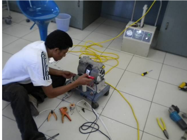
Cesar Augusto rebuilds a suction pump in Timor-Leste
