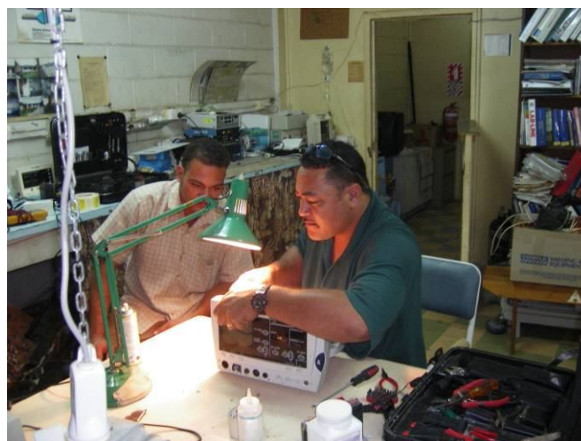
Samoa BMETs repairing a patient monitor
