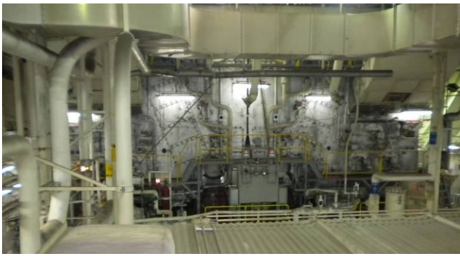
The Engine Room- Two massive boilers driving two turbines and a single prop shaft
