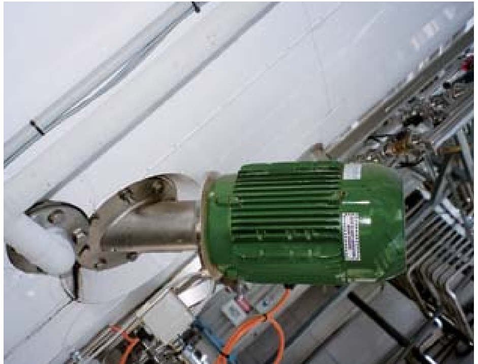
Mixquip agitators are now fitted with a mechanical seal.
