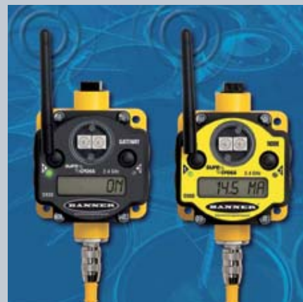
Nodes (right) send information to the gateway (left).
