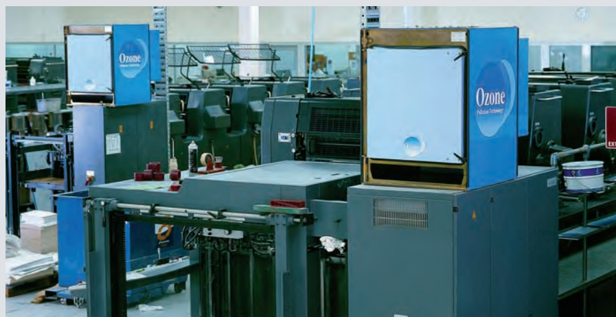
Ozone gas cleaners are suitable for cleaning the ambient air in a workshop.
