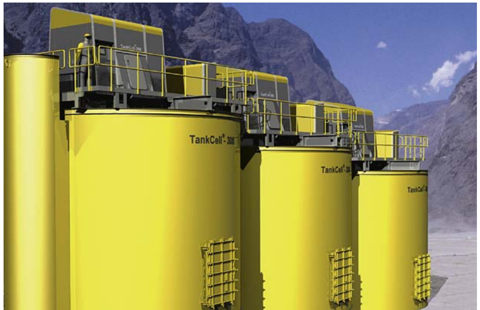
Rendering of the new large mechanical flotation cells to be installed at Oceanagold's Macraes mine in New Zealand.
