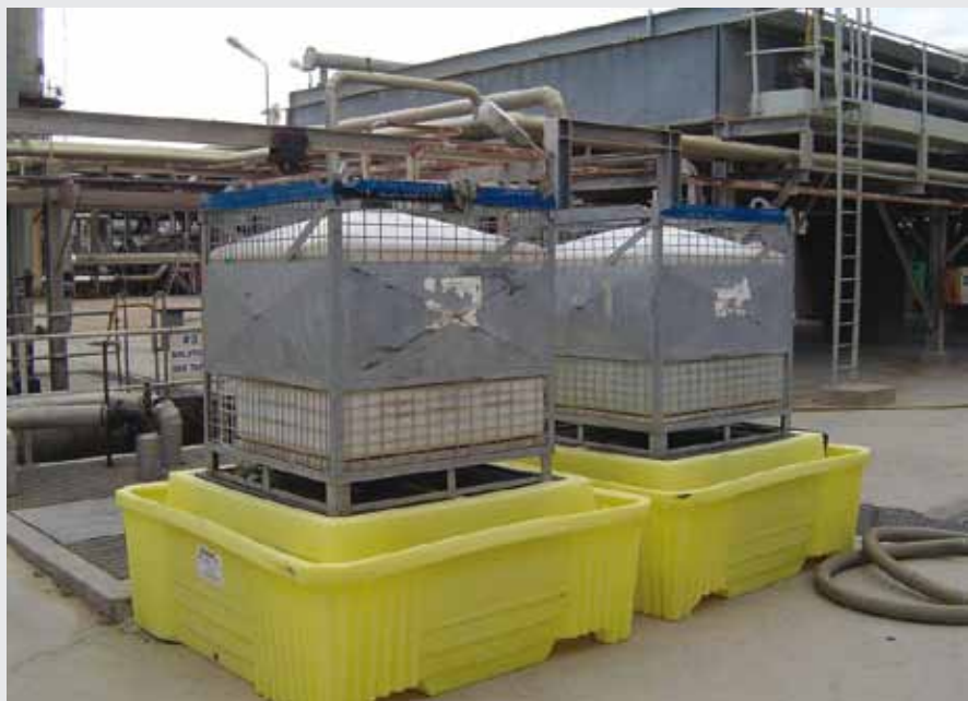
The IBC 2000i spill containment unit can fit a 1000L container.
