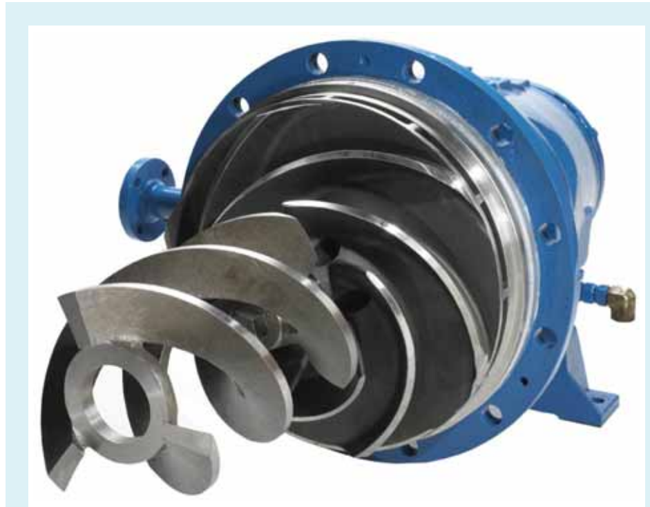
The Gould Pump agitates paper pulp to assist flow.
