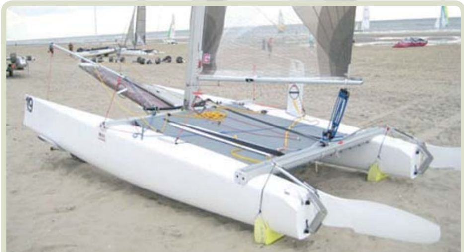
The hull of the completed boat was accurate to within half a millimetre.
