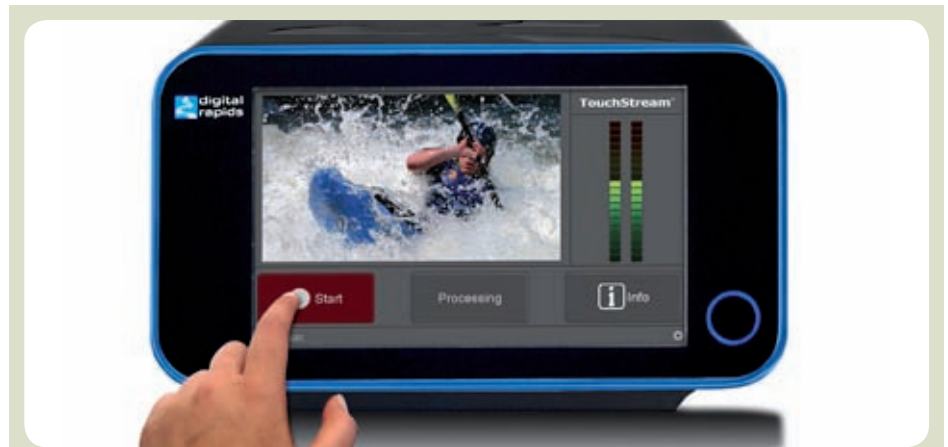
The unit has a touchscreen interface with integrated live video monitoring.
