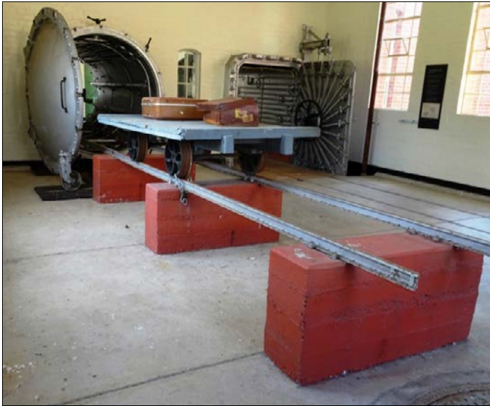
Luggage on an elevated trolley about to enter the steam chamber. The door to the disinfecting chamber can be seen behind the luggage trolley. Ph: K. Baker.
