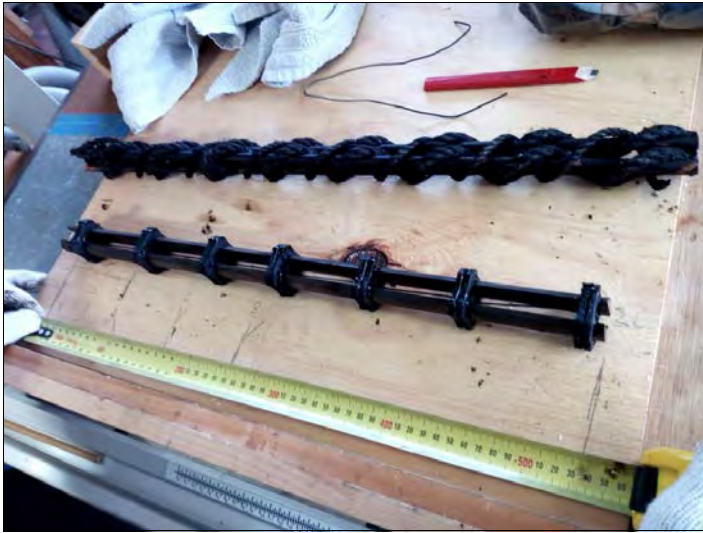
Above: Sections of 2-core (bottom) and 3-core (top) conductors and separators removed from pieces of Edison Street Tubes to prepare for display.
