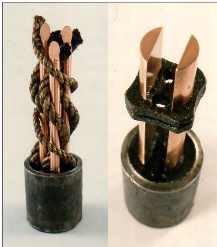
Cut-away examples of the 3-core (1892) and 2-core (1884) Edison Street Tubes recovered in 1992, showing the internal construction as described at right.
