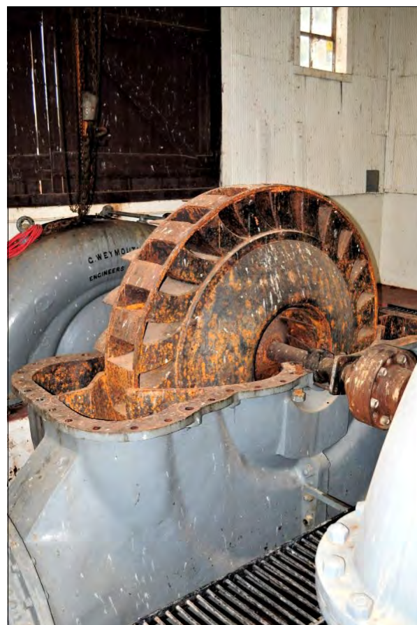
Image above: A Weymouth centrifugal pump with the top removed. Photo: Owen Peake.
