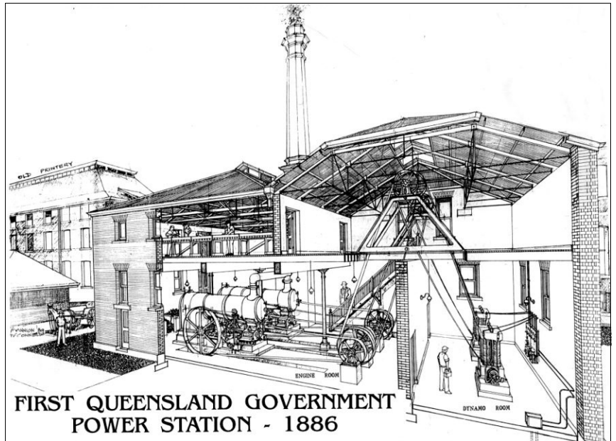
A recent cutaway drawing shows the Engine Room at left and Dynamo Room at right. Image: source not provided.
