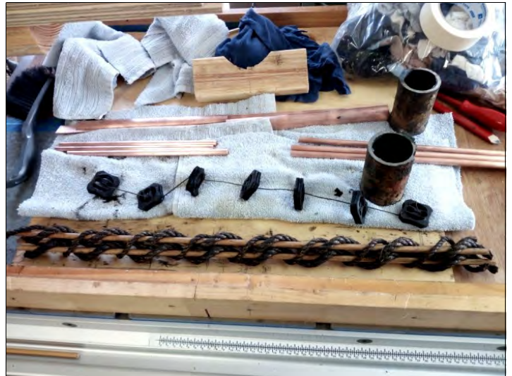
Right: Copper conductors and separators/insulation disassembled and cleaned in preparation for making up a display like the one below.
