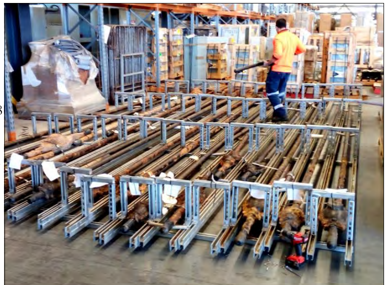
Above: Recovered Edison Tube lengths with joint “boxes” in special frames ready for transport.
