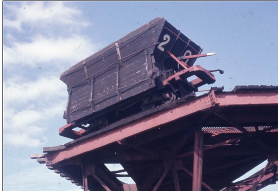
Empty No.20 hopper car turning at the end of the pier to return to the tunnels for re-filling. Source ARHS Collection - no date.
