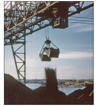
Detail of photo showing a grab bucket releasing its coal onto the stockpile. This post WW2 gantry crane replaced the two originals. Photo, Patrick Trevor. Source: NSC
