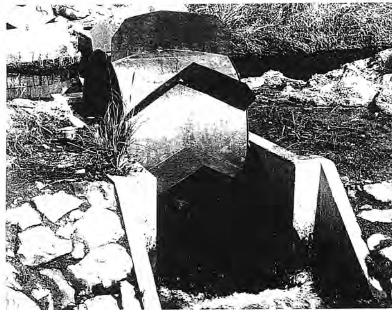
A Dethridge wheel metering water at farmer's supply point
