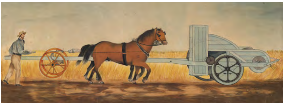
Ridley's first Stripper – the horses are pulling a crossbar connected to a beam which pushes the machine ahead of them [State Library of SA SRG 112]
