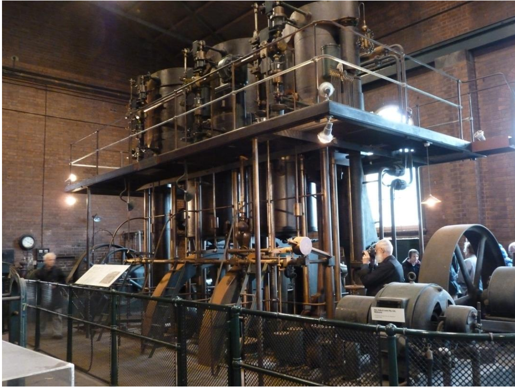
Hathorn Davey steam pumping engine at Spotswood. Image: Miles Pierce
