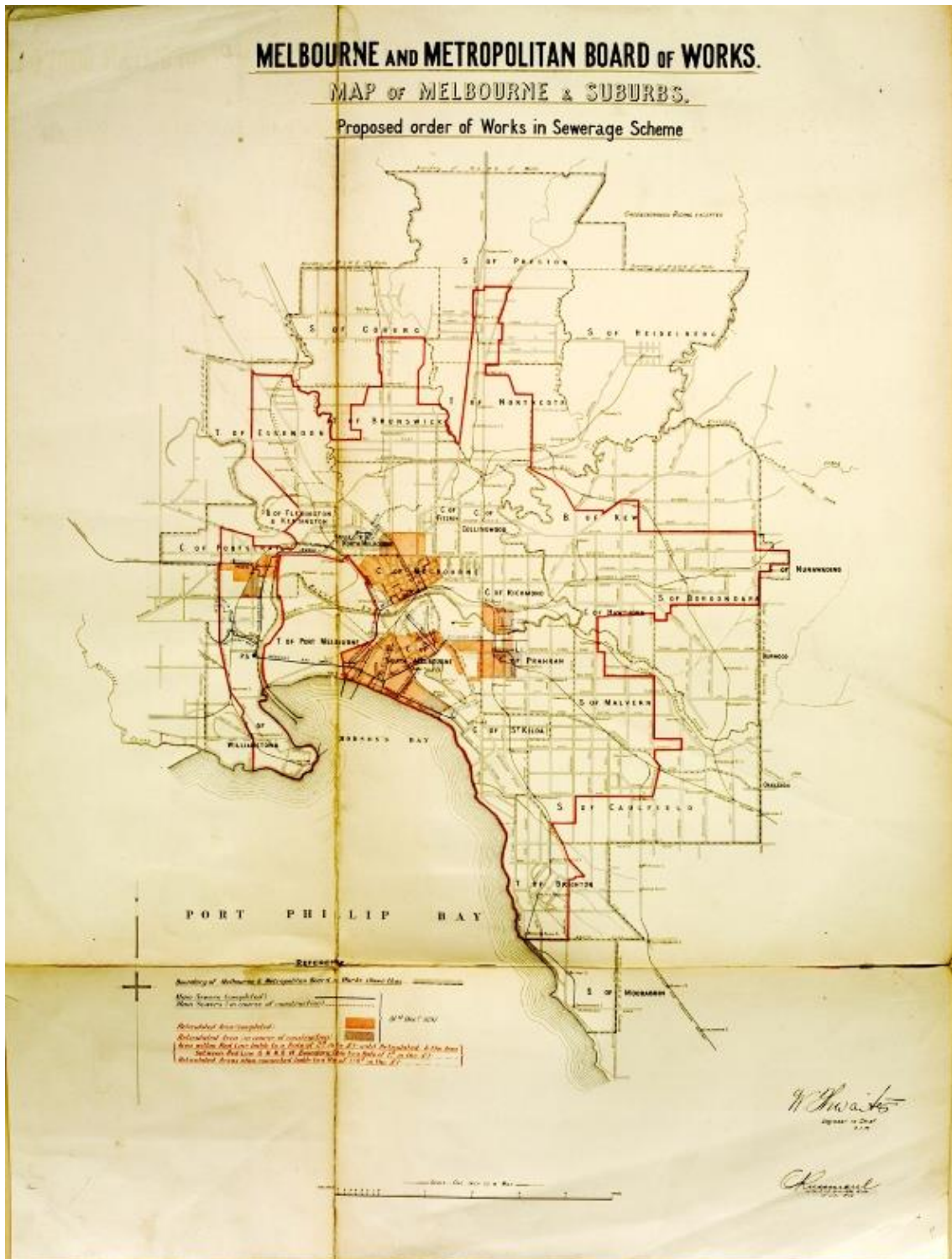
Map of Melbourne showing extent of the sewerage system completed or under construction (coloured areas) in 1897. Note that the map is signed by William Thwaites. Image: Culture Victoria
