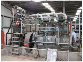
This 132 bhp (98kW) engine (no.154551) was built in 1929 and installed in the AMP Building, at the corner of Collins & Market Streets, Melbourne as a standby generator. It is a 4VXC model, and illustrates the earlier form of engine construction with separate cylinders. The engine is directly coupled to the DC generator and also drives via belts an AC alternator. It is historically significant as an example of the first generation of large industrial diesel engines installed in Melbourne.
