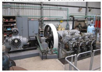
network of ship fuelling ports. The Guinard variable displacement pump built by Stothert & Pitt, Bath, England is technically significant, and this is a large example of its type. The internal complexity
