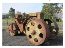
Melbourne. The fifth is an example of an 8 ton roller built by Malcolm Moore Pty Ltd, Port Melbourne which was originally owned by the Country Roads Board.
