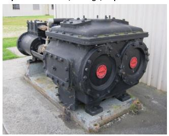
Two large horizontal Worthington type duplex pumps were supplied c.1917 to the HMAS Cerberus naval base at Flinders. These pumps were used to transfer bunker fuel to storage tanks at the base. They are significant as rare examples of machinery built by Taylor Horsfield in Bendigo. They are technically significant as large examples of their type, and for their application for pumping bunker oil. The photograph shows one of these pumps.
