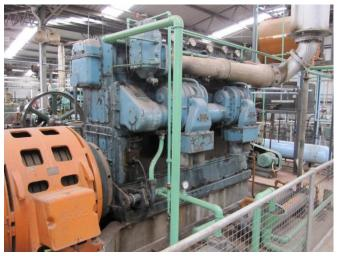
effect assists the flow of a fresh fuel-air mixture charge into the cylinder. The engine illustrates the intermediate stage of engine development prior to turbo charging with the application of mechanical supercharging.
