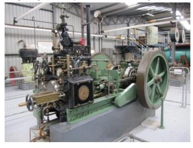
tachometer, thermometers, and engine indicators to allow the study of engine efficiency under various conditions. It is a rare operational example of an engine specifically built for teaching, and demonstrates an important aspect of the earlier training methods used for mechanical engineering students.
