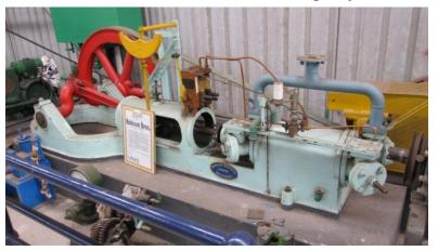
This single-cylinder horizontal reciprocating compressor was made by Robison Bros. in South Melbourne, and most likely dates from the early 1890s. It was acquired by Swinburne University and converted to an air compressor, and used for teaching engineering students. It is a very rare early example of an Australian made refrigeration compressor.
