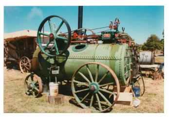
The Johnson portable steam engine is a rare example of a Victorian built portable steam engine. This example was built c.1895-1910 for the Victorian Mines Department, and was used at the Queenstown state battery. It appears that the Mines Department owned several of these engines, and they were used at various state batteries. It is fitted with a single cylinder engine mounted on a cylindrical Jackass boiler. It is the only example known to be in complete condition.
