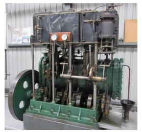
This compound marine engine with surface condenser was built in the 1890s by D. & R. Buchanan. This firm of marine engineers were based on the banks of the Yarra River in South Melbourne, and it is known that they built several engines of this size for Victorian Defence Department launches. The engine was later used at the Engine Driving school at RMIT before being purchased for the collection in 1969.
