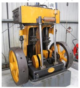
This compound vertical open crank engine is a rare example of a steam engine built by Kelly & Lewis, at their Melbourne factory. The provenance of this engine is not known. It is an early example of an engine made by Kelly & Lewis from the steam period. The firm was better known for their later production of oil engines, Bulldog tractors, and centrifugal pumps and air compressors. The engine is on long term loan to the museum.
