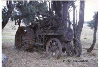
technically significant as one of three known examples fitted with Joy valve gear. The engine is also representative of the many traction engines used for chaff cutting and threshing on farms around Australia.
