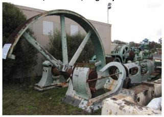
This compressor was one of two installed in the engine room of the Victoria Brewery of Carton & United Breweries Ltd. (CUB), Abbotsford. It was driven by electric motor via a rope drive and was rated at 100 tons capacity (i.e. 100 tons of ice in 24 hours). It is an important example of a locally produced compressor, and was amongst the largest built by Werner. It is also representative of the use of refrigeration in the brewing industry, and significant for its association with CUB.
