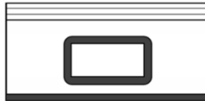
Diagram showing residual section after char around a penetrated primary beam.
