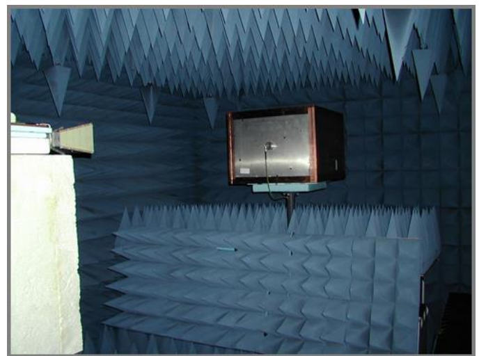
Figure 12 Enclosure in NIST anechoic chamber
