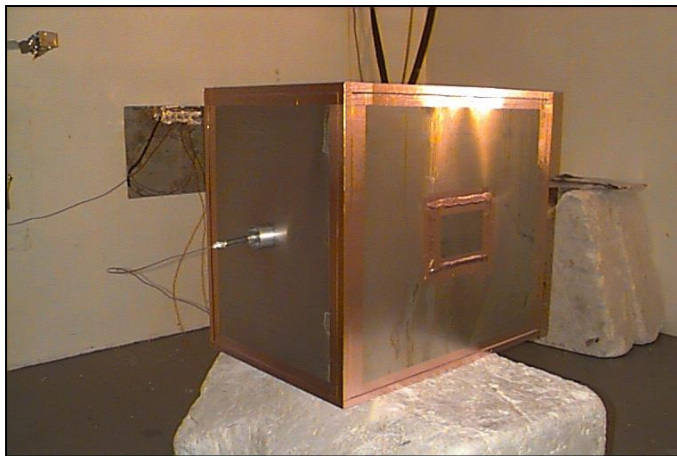
Figure 9. Shielded enclosure in NSWCDD reverberation chamber
