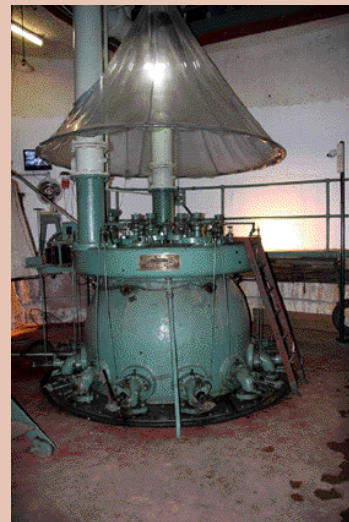
The combustion head of the Humphrey pump
