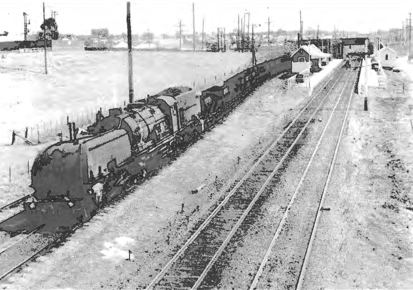
Garratt Locomotive 6002 hauls coal from Liddell Colliery through Tarro on one of the two special coal tracks which were installed early this century.
