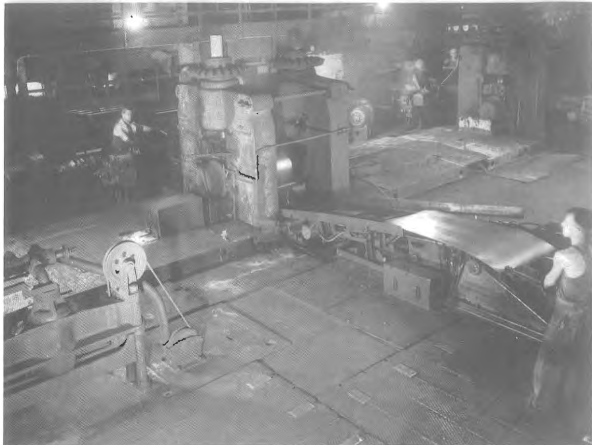
Workers turning a "pack" in the manual rolling operation at Lysaght's. JL
