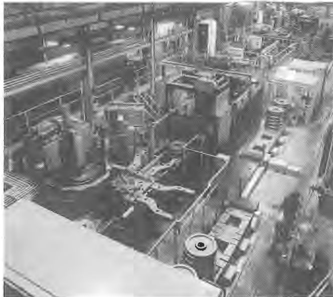
Pictured operating at the Commonwealth Steel Works, the new computer-controlled automatic wheel-turning machine. CS
