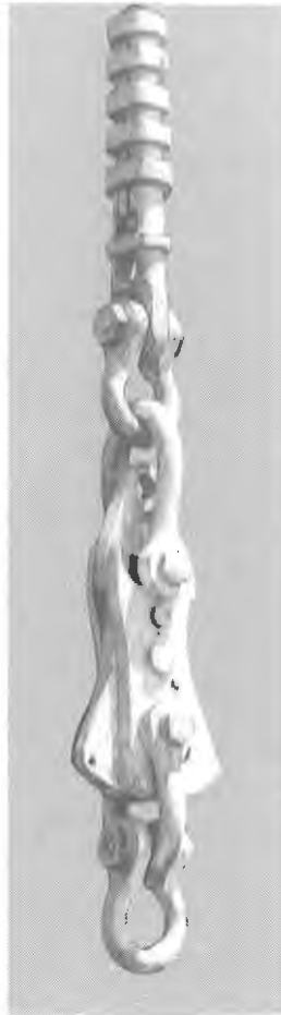
An Ormerod mine cage detaching and suspension gear. This kind of job is a speciality of Hexham Engineering. HE
